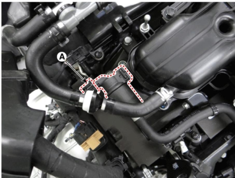
3. Disconnect the vapor hoses (A) from the purge control solenoid valve.
